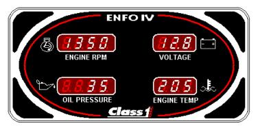
If CAN information is not present the Engine RPM, Oil pressure, and Engine temp displays will flash the CAN ERR message.
