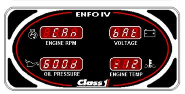
*Indication of CAN invalid and 24V ignition system detected* →
